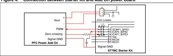
Figure 4. Connection between Starter Kit and Add On power board
