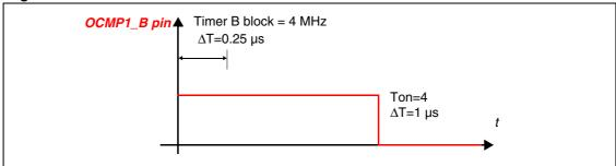
TimB\_init (Ton) is used to set up the Timer B to generate the pulse. Ton sets the number of steps of the timer in which the timer output is high.
