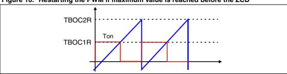
Figure 10. Restarting the PWM if maximum value is reached before the ZCD
