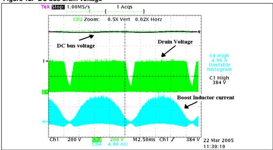
Figure 13. Characteristics of drain voltage and inductor current
